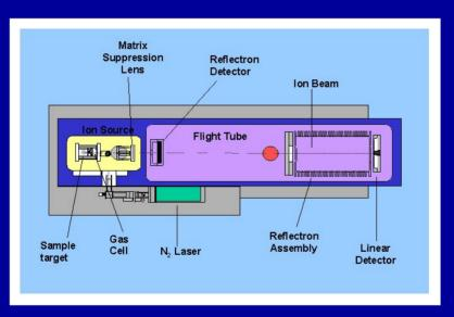
Differentiates particles with different masses by their travel time in the tube.
